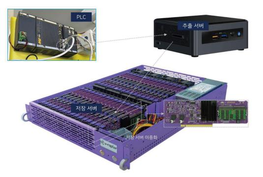
We have built a private cloud that can extract and store data within the factory in real time and share it with the outside without reinforcing separate cooling and power facilities.
