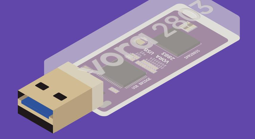
And, we are making ultra-small edge AI products. The GTI SPR2803S NPU mounted here boasts **16.8TOPS** performance **at 0.7W** ultra-low power. **Edge Al**
