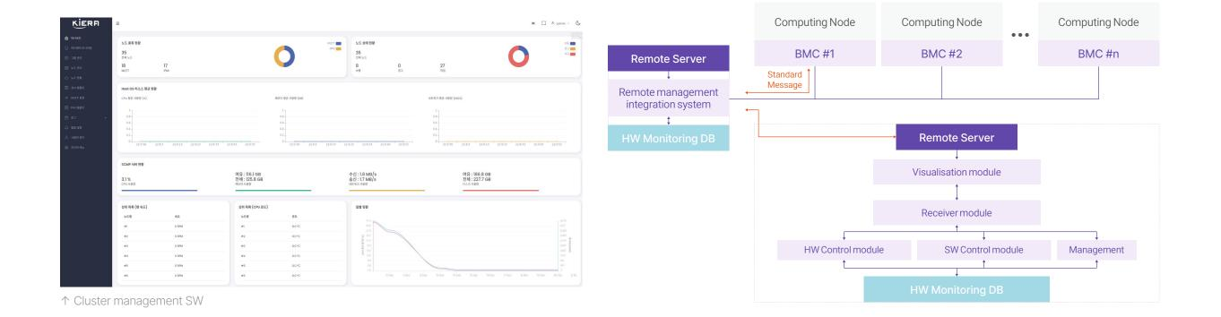
KiERA is a SW developed to remotely monitor and manage the hardware functions of high-performance server nodes, collect, analyse, and manage the status information of each node's hardware based on BMC, and perform efficient remote processing.
